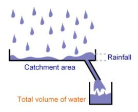
Volume of Rainfall per Hour (litres) = Precipitation Rate per hour (mm) X Area (m<sup>2</sup>)
